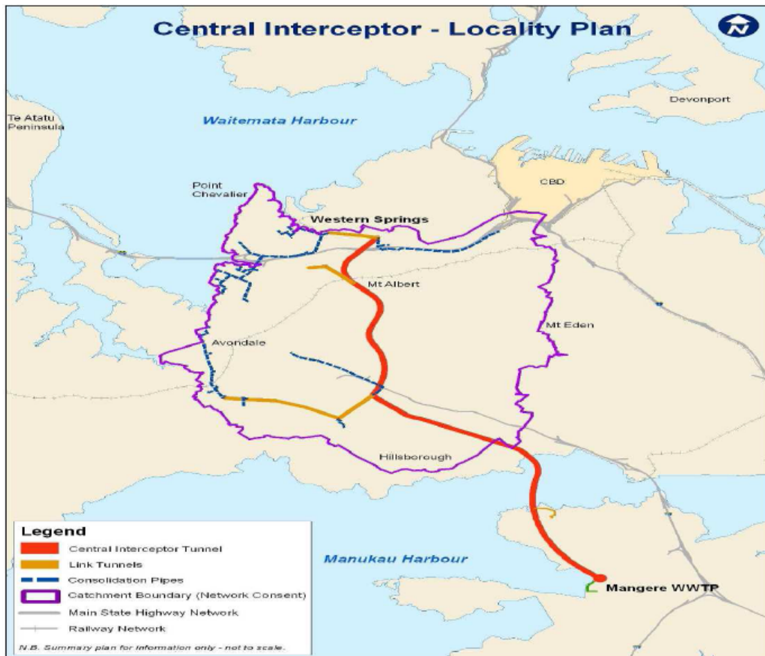
Figure 4 Proposed Central Interceptor which would pipe sewage away from Western Springs and surrounding suburbs to Mangere for treatment.
